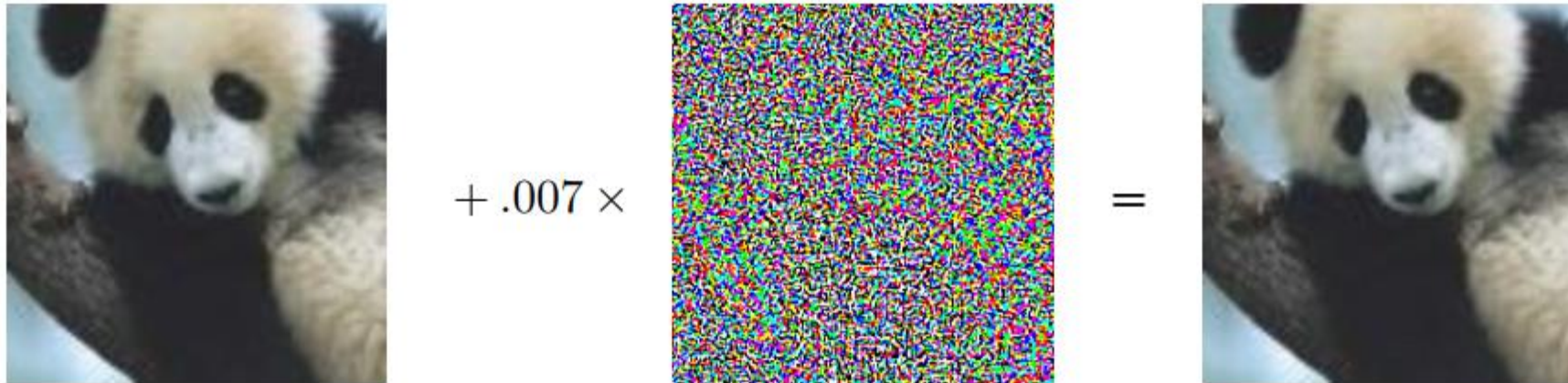
Figure 2: Illustration of adversarial sample generation using a disturbance vector weighted by a scalar value of 0.007. The "benign sample" (left) was originally classified as panda with 57.7% confidence, but the adversarial sample (right) was classified as gibbon with 99.3% confidence.
